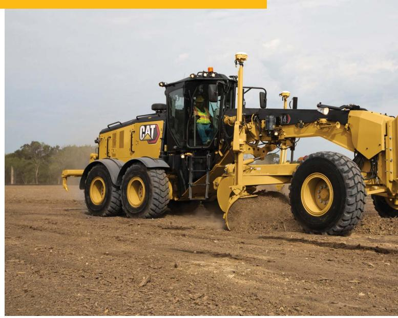
The front axle steering cylinder and sensing guards have been designed to enhance durability and hydraulic hoses have been routed to improve reliability.
