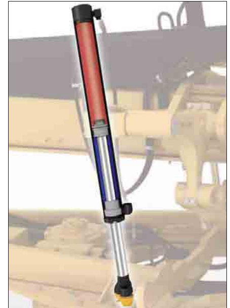
Scharhubzylinder: rot = 40 l/min, blau = 24 l/min
